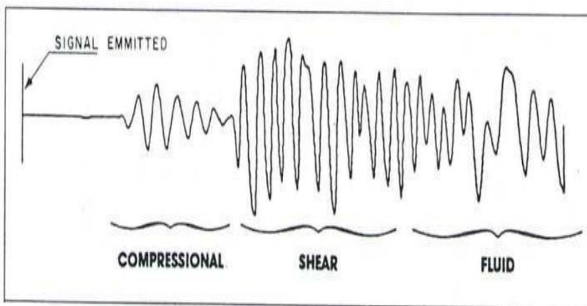
Figure 2: Typical sonic waveform in borehole [9]
