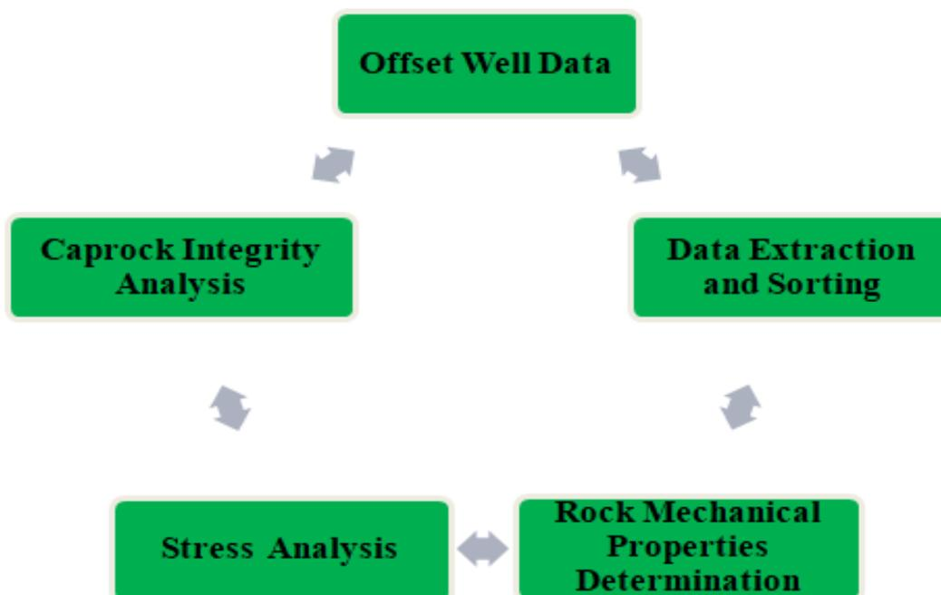
**Figure 3: Workflow for Geomechanical Analysis**
