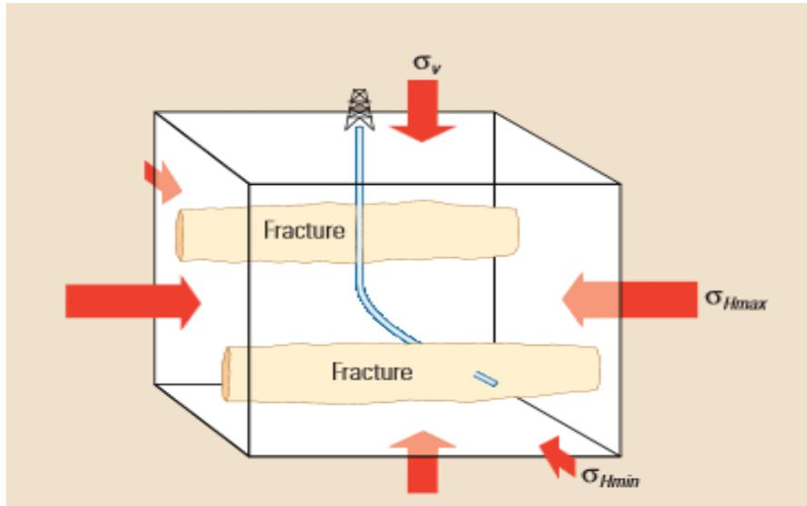
Figure 5: In-situ stresses and fracture orientation [13]
