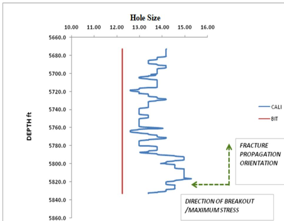
Figure 6: Fracture Propagation Orientation for field X
